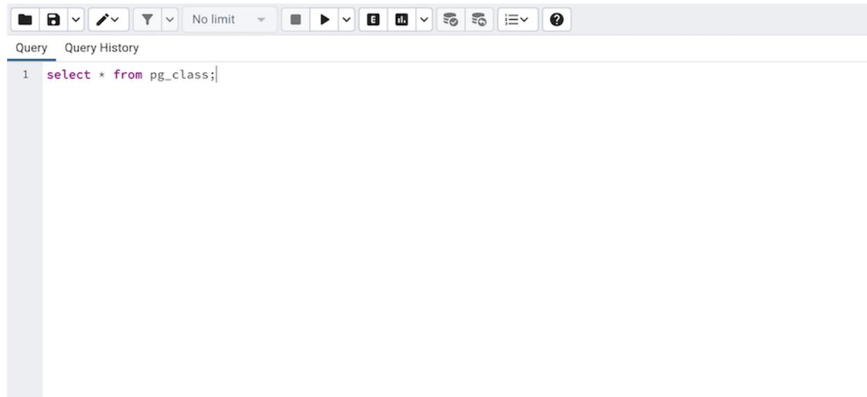
To use autocomplete, begin typing your query; when you would like the Query editor to suggest object names or commands that might be next in your query, press the Control+Space key combination. For example, type “*SELECT \* FROM*” (without quotes, but with a trailing space), and then press the Control+Space key combination to select from a popup menu of autocomplete options.
