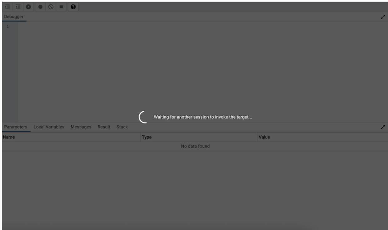
When another session invokes the target, the debugger will display the code, allowing you to add break points, or step through line-by-line. The other session is suspended until the debugging completes; then control is returned to the session.
