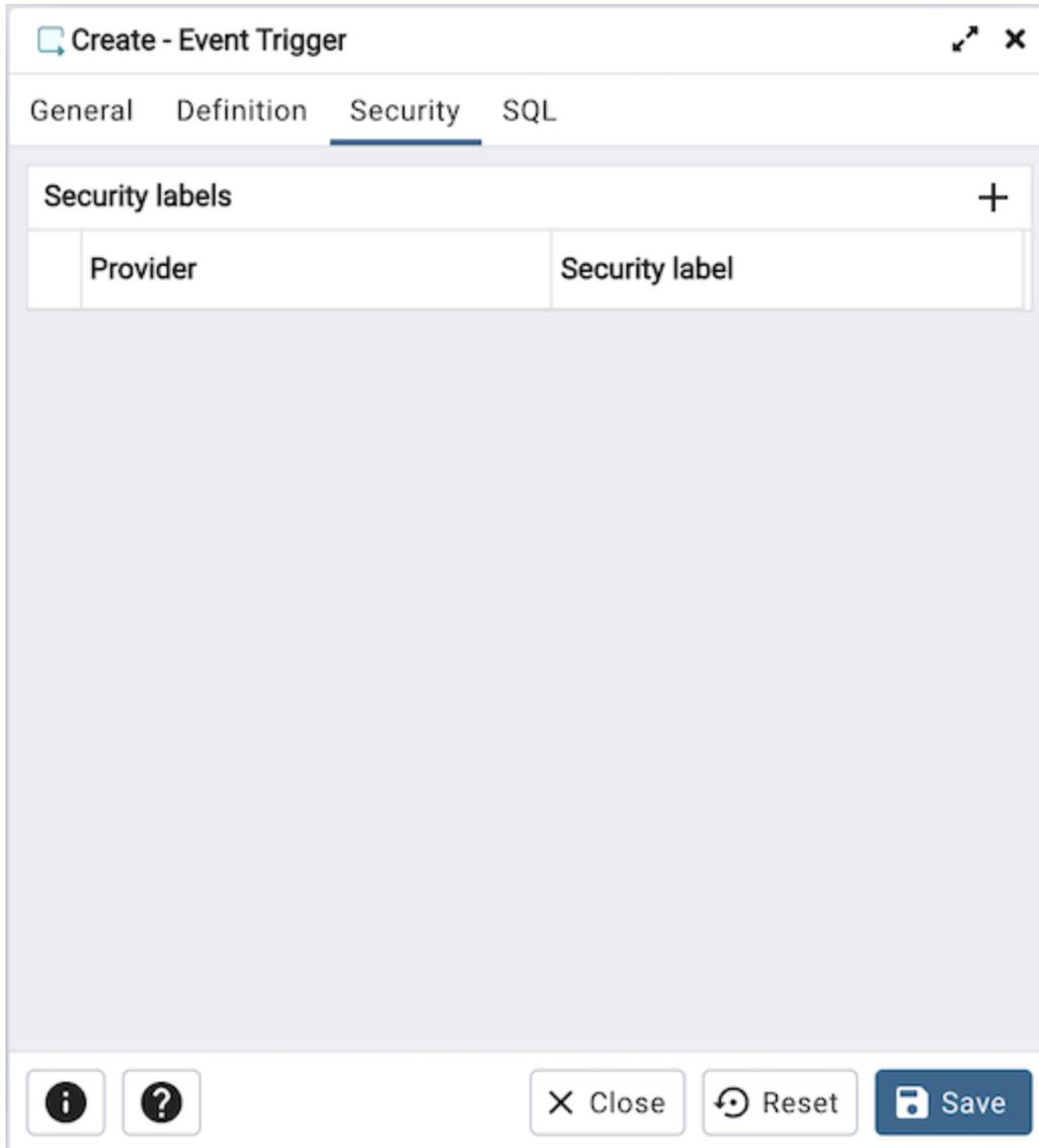
Use the *Security* tab to define security labels applied to the trigger. Click the *Add* icon (+) to add each security label.
