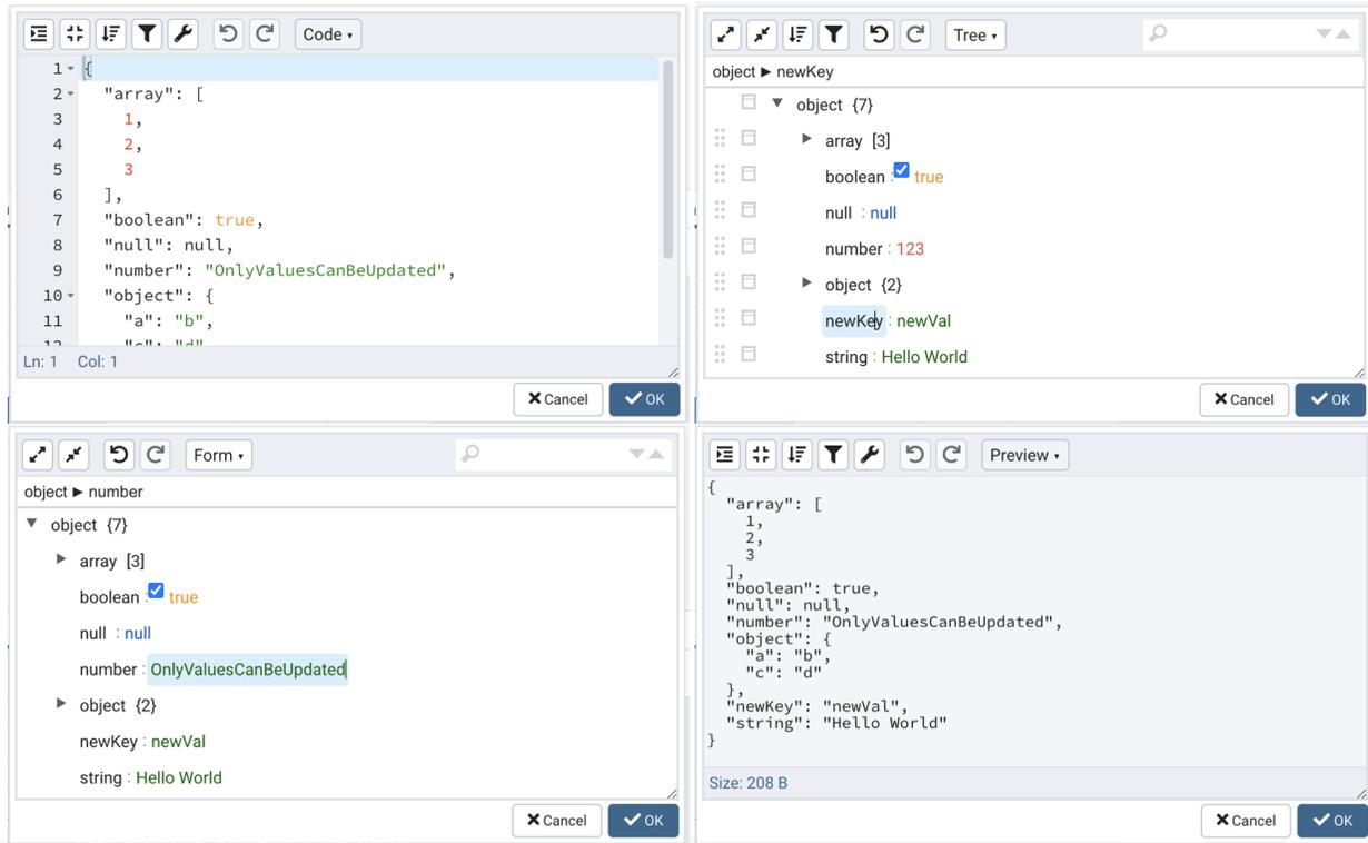
**Code Mode:** Provides way to format & compact json data. Also provides ability to repair json data by fixing quotes and escape characters, removing comments and JSONP notation and turn JavaScript objects into JSON.
