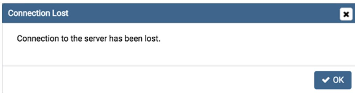
This error message indicates that the connection attempt has taken longer than the specified threshold; there may be a problem with the connection properties provided on the *Server* dialog, network connectivity issues, or the server may not be running.
