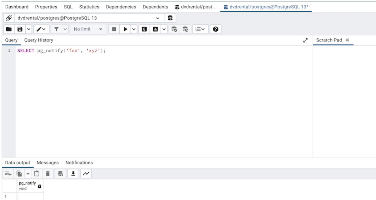
3. You can observe the *Notification* tab in the first *Query Tool* session where it shows the Recorded time, Event, Process ID, and the Payload of the particular channel.
