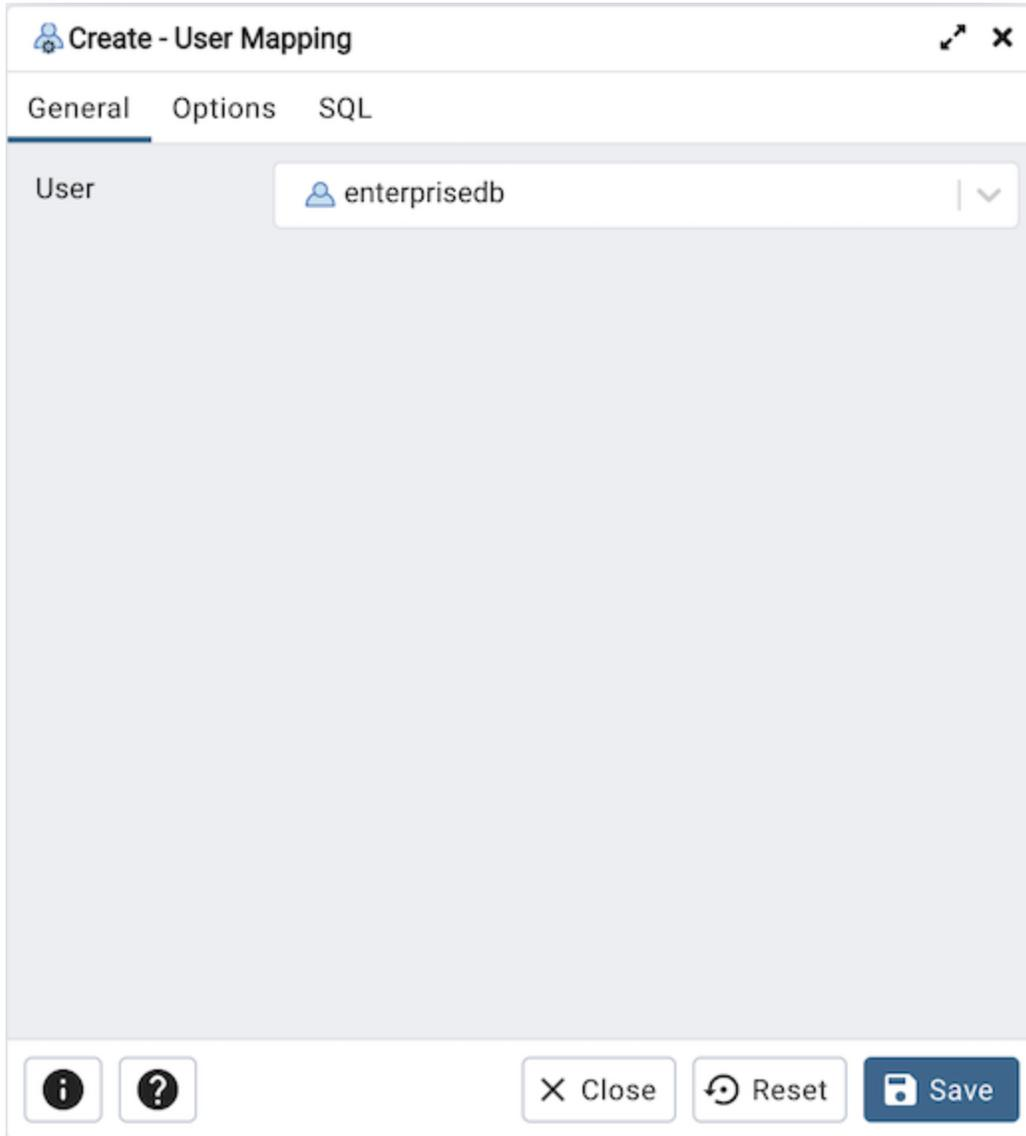
Use the drop-down listbox in the *User* field in the *General* tab to identify the connecting role:
