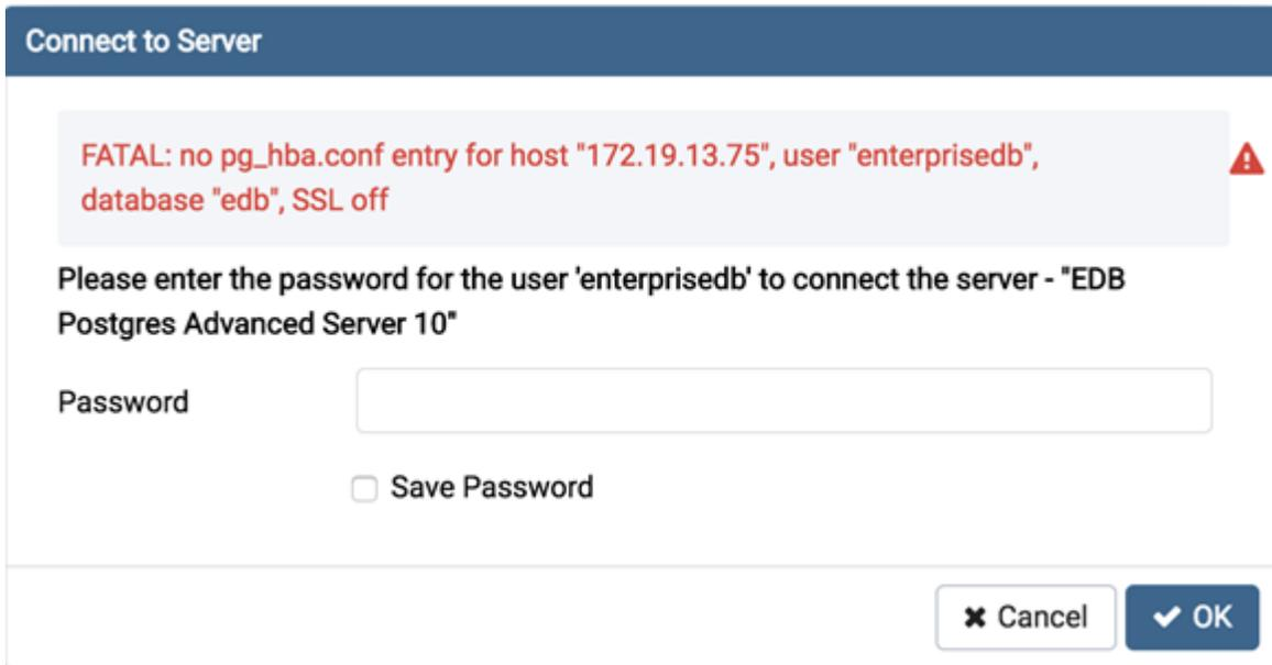
If pgAdmin displays this message when connecting, your server can be contacted correctly over the network, but is not configured to accept your connection. Your client has not been detected as a legal user for the database.
