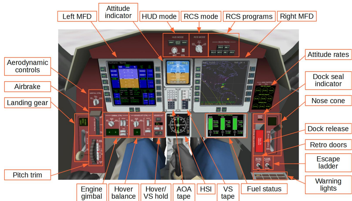
Delta-glider virtual cockpit: main instrument panel
